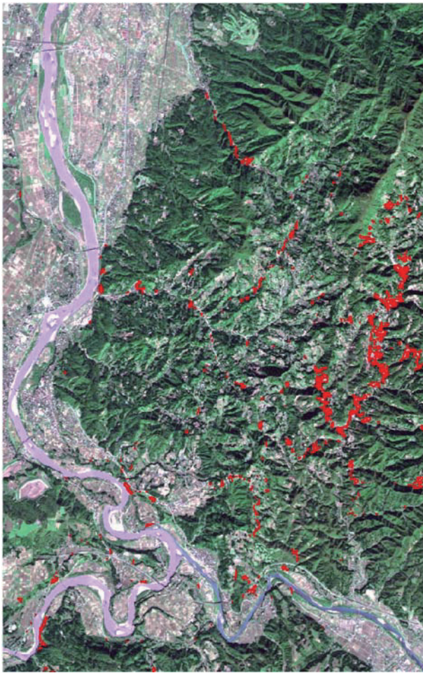
Figure.6 Detected damage area by NDVI analysis Red polygon : detected damage polygons (background image : SPOT-5)
