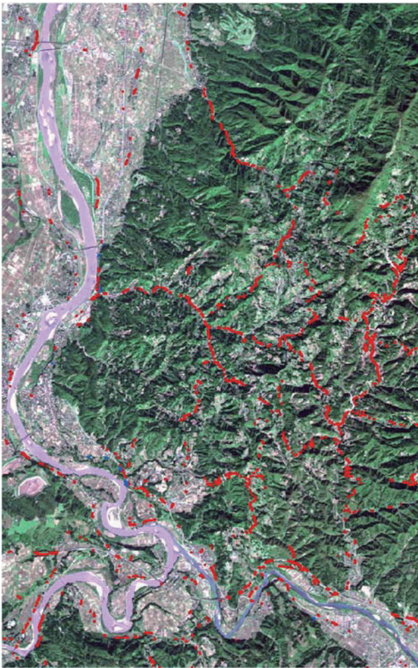
Figure 9. Post processed (merged) damage area Red polygon : damage of road Blue polygon : damage of railway
