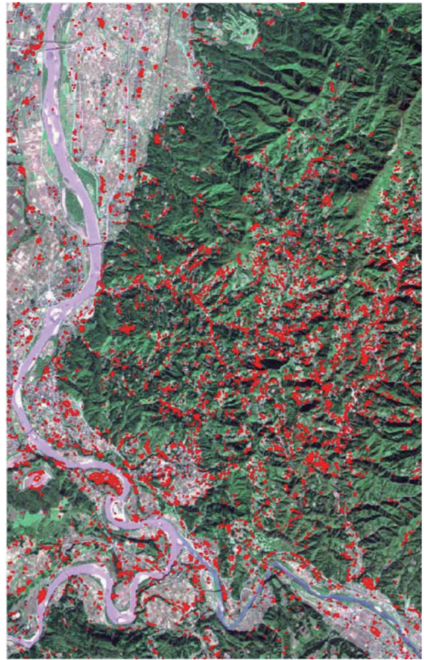
Figure 8. Detected damage area by texture analysis Red polygon : detected damage polygons (background image : SPOT-5)
